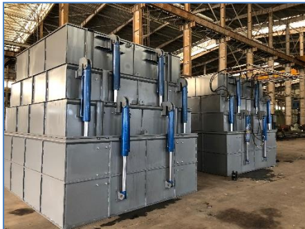
Automatic coal discharge system
